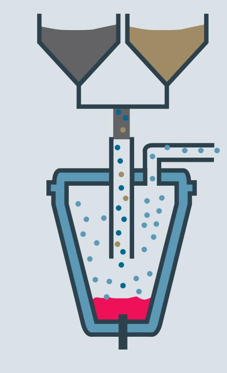
HYDROGEN PLASMA SMELTING REDUCTION replacing coal
